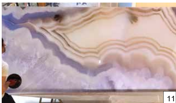
Posa lastra GemGlass su pannello LED Mounting GemGlass slab on LED panel
